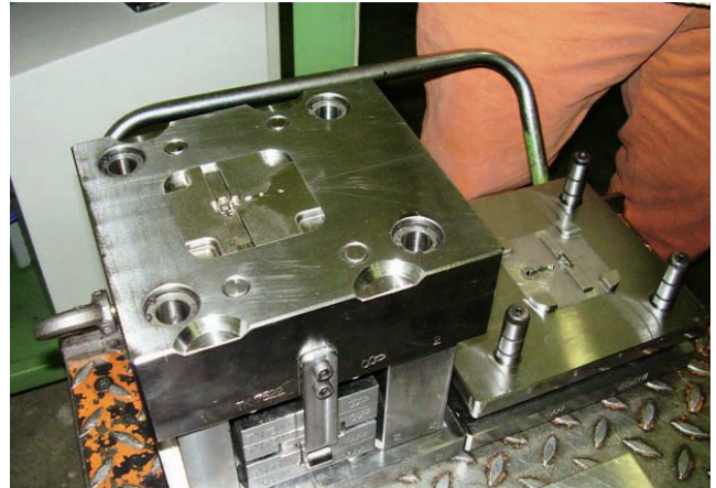
Cobalt Chrome tool with conformal cooling channels, in production in an injection moulding machine at BTicino.
